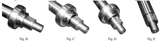
**9.** Loosen the two (2) set screws in each of the bearings, and slide them off. If the bearings are too tight to slide off, use a gear/pulley puller. <u>Do not use a hammer or any other blunt force object to "work" the bearing off of the shaft</u>. If the shaft becomes damaged, it may need to be replaced.
